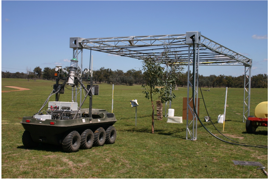
Figure 15: Static test area with radar reflectors (Datasets 22 & 23)
