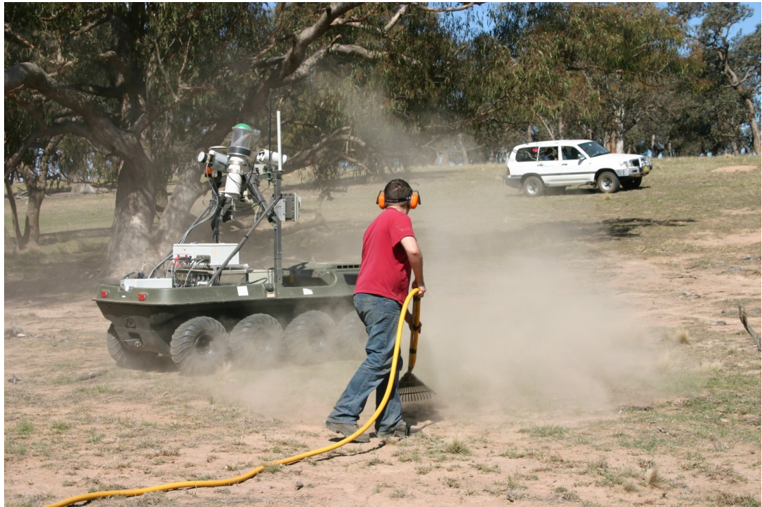
Figure 21: Dynamic test in the dam area with dust (Datasets 36 to 37)
