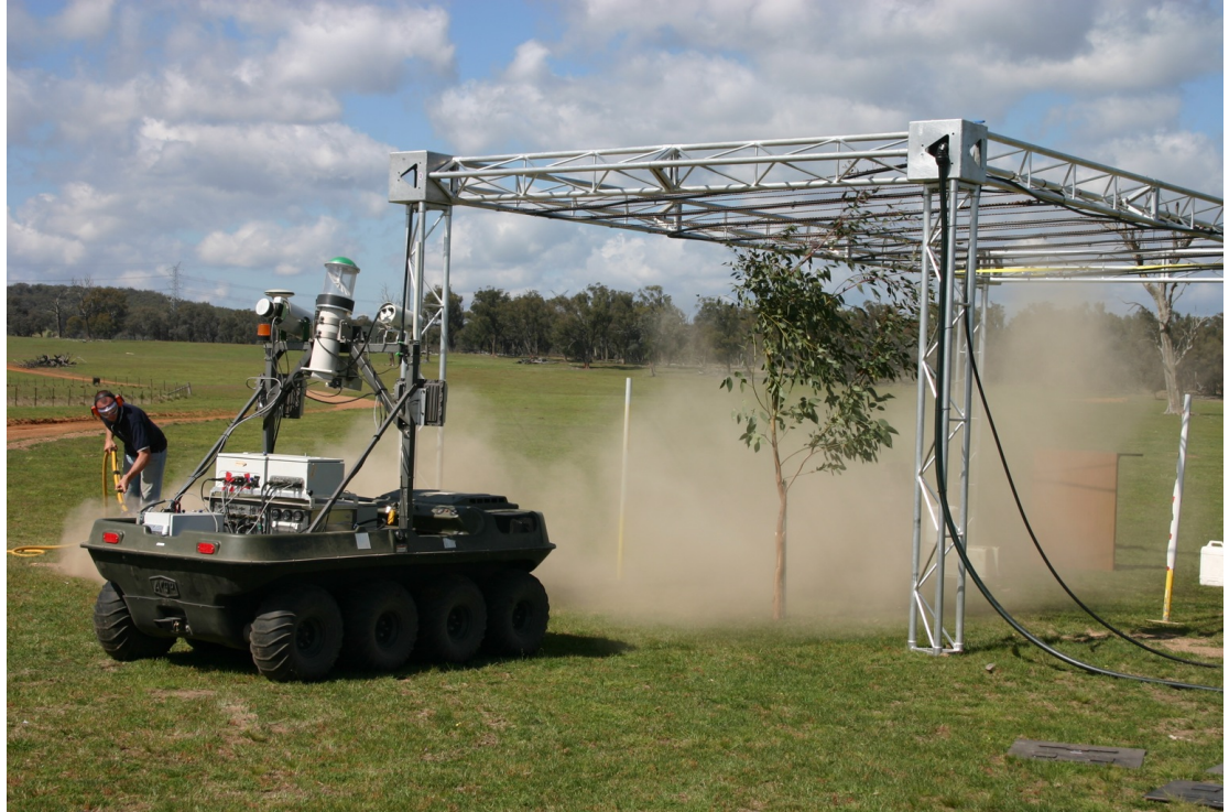
Figure 12: Static test with heavy dust (dataset 15)
