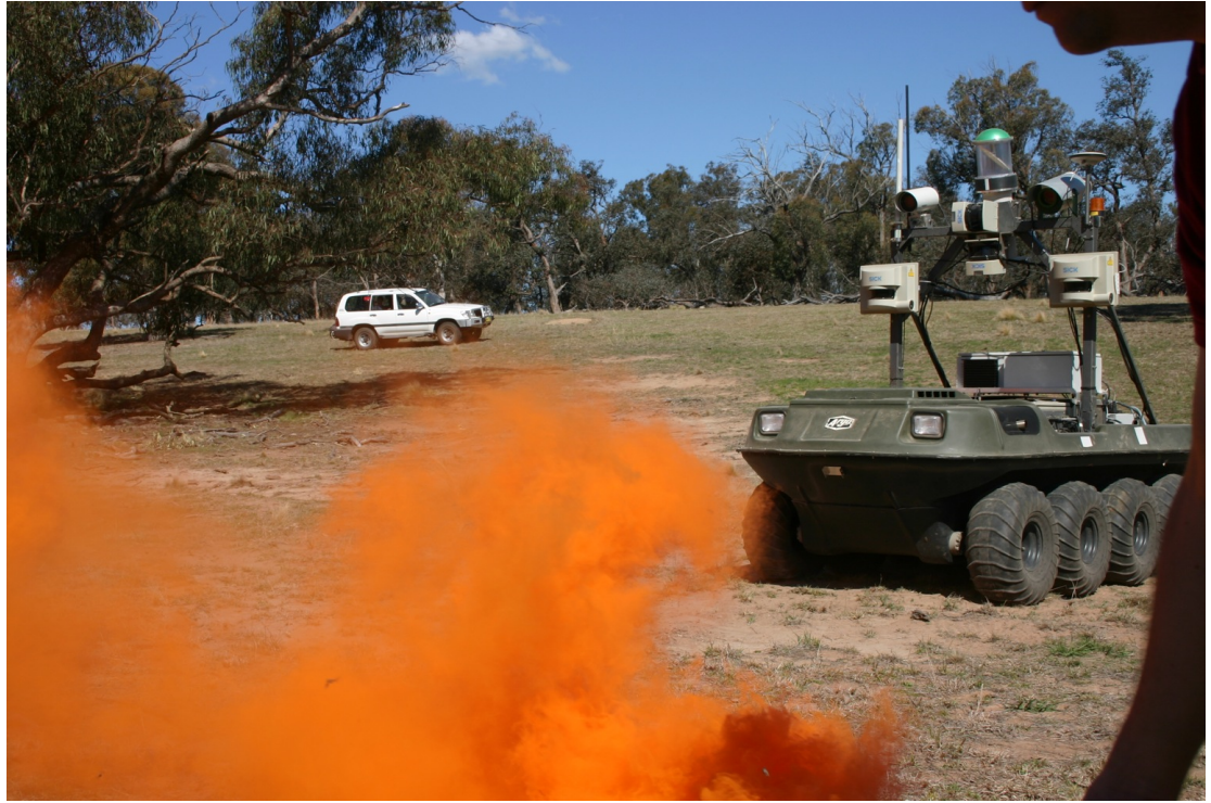
Figure 22: Dynamic test in the dam area with smoke (Dataset 38)
